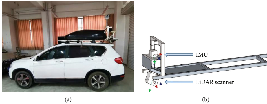
FIGURE 1: The integrated spatial geometric position relationship between the LiDAR sensor and the IMU of the VLS system. (a) The self-developed VLS system is shown. (b) The geometric position and coordinate system of the LiDAR scanner and the IMU are shown, in which red represents the X-axis, blue represents the Y-axis, and green represents the Z-axis.
