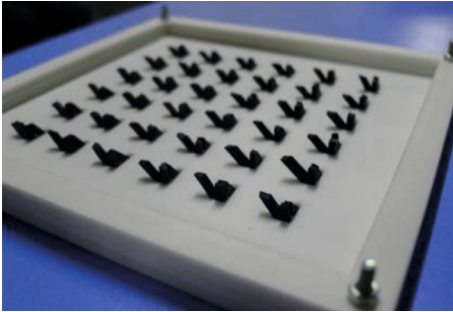
FIGURE 2: 3D printed mold with 6 × 6 sensitive elements.
