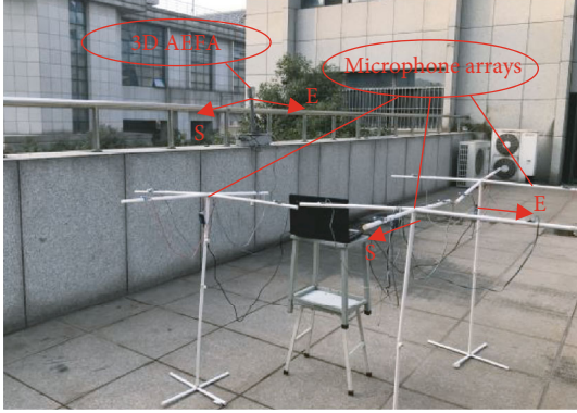
FIGURE 11: Arrangement of AEFA and microphone arrays.
