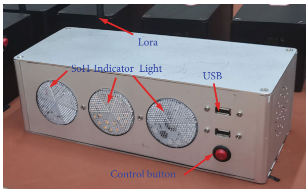
FIGURE 4: Intelligent control warning node.
