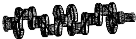
Binarization result of crankshaft structure in stl format
