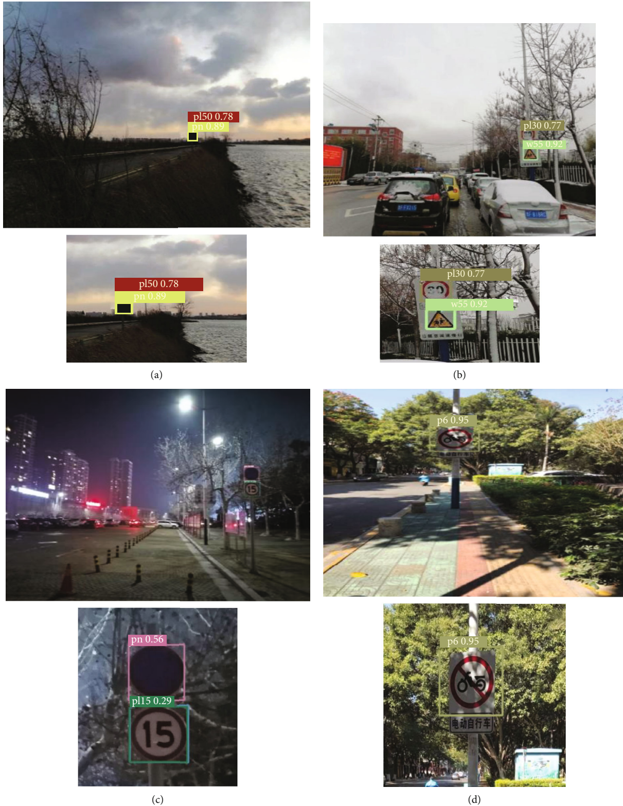
FIGURE 15: Street view images and detection results from TS-Yolo. ((a) Cloudy; (b) snowy; (c) dimly at night; (d) shadow occlusion).
