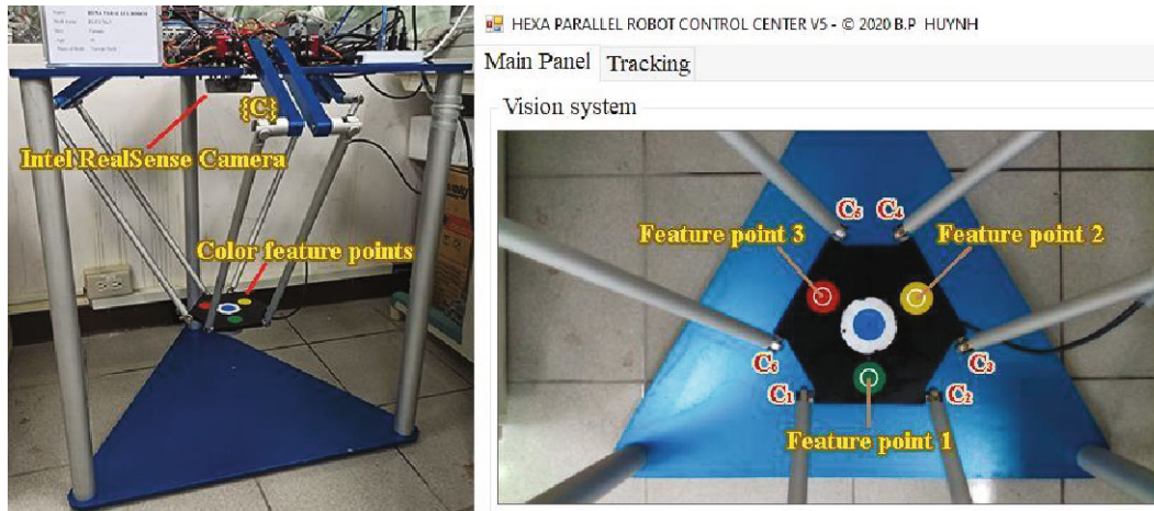
FIGURE 3: The vision system of the real robot (a) and the vision system on the control software (b).
