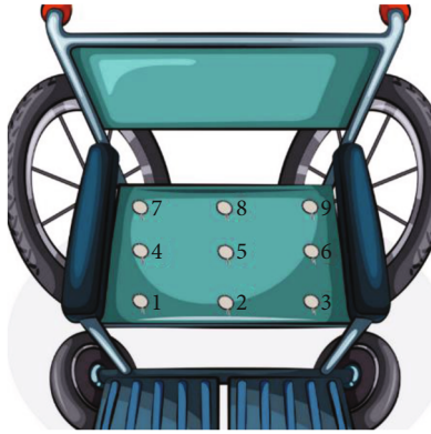
FIGURE 2: 3 \times 3 matrix sensor configuration.
