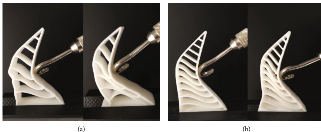
FIGURE 15: Fingers bear 10 N load: (a) six-rib finger structure; (b) ten-rib finger structure.
