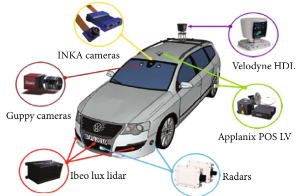
FIGURE 2: Sensor set-up of MadeInGermany. Externally visible part of sensors [9].
