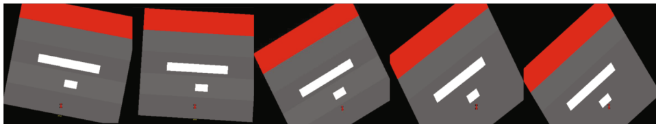
FIGURE 5: An episode in training, with the obstacle in white, the end of the road in red, and the viewpoint following the Agent, where the car hit the obstacle, terminating this episode.
