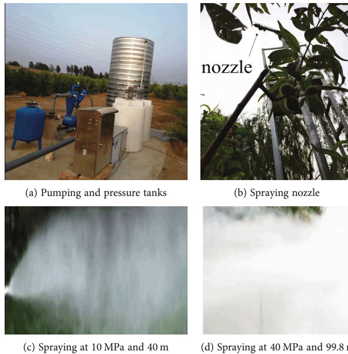
FIGURE 6: The spray water fog effect with different pressure and range.
