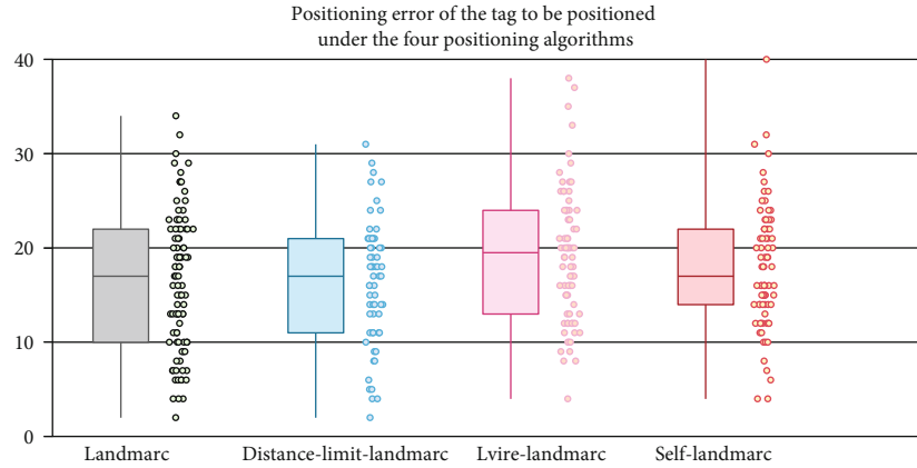
FIGURE 5: Positioning error of the tag to be positioned under the four positioning algorithms.
