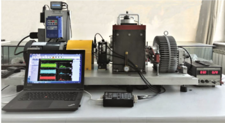
FIGURE 7: Comprehensive test bench for power transmission fault diagnosis.
