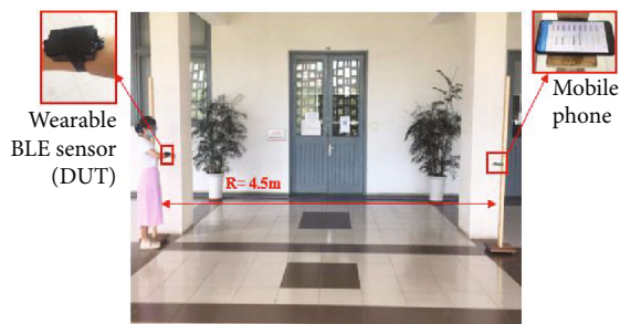
FIGURE 17: Read-range measurement of U-shaped monopole integrated antenna in wearable BLE sensor.
