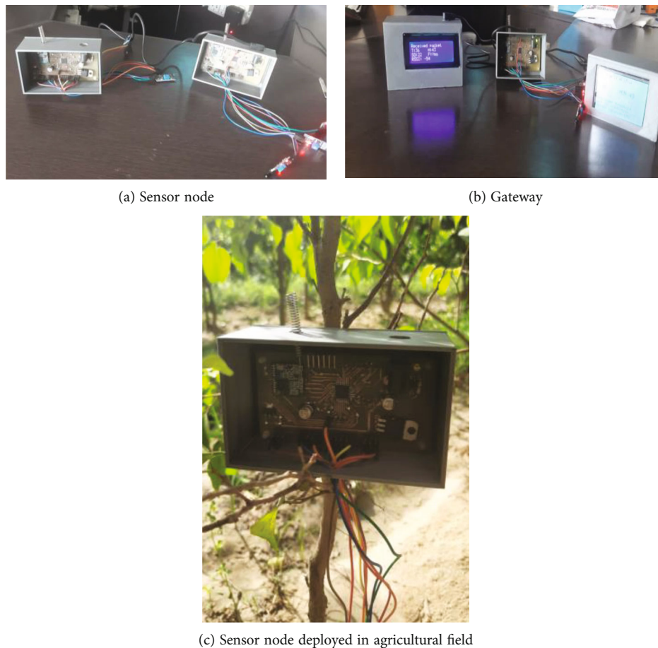
FIGURE 11: Final hardware and deployed sensor node in the agricultural field.
