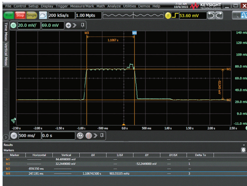
FIGURE 15: Voltage of eMeD during active and idle modes with event-driven management algorithm.
