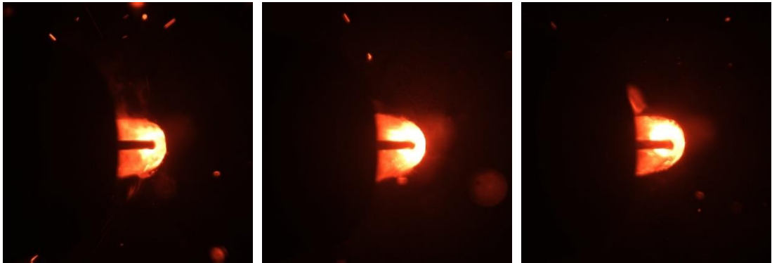
Figure S1: Test images at three typical moments under the process conditions of 95A, 19V, and 23cm/min.
