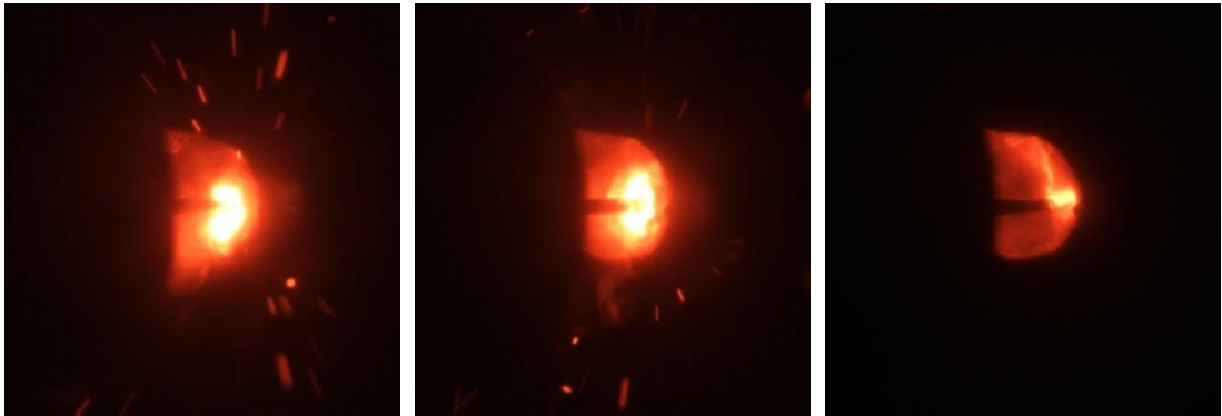
Figure S10: Test images at three typical moments under the process conditions of 150A, 21V, and 26cm/min.
