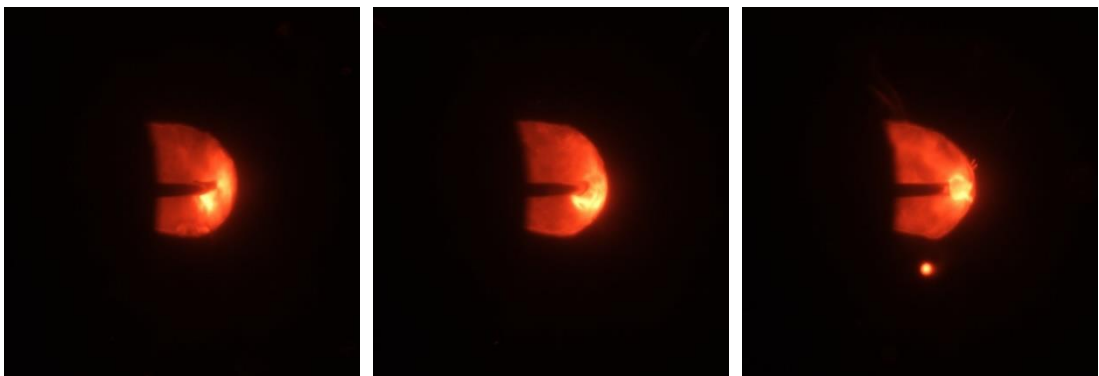
Figure S6: Test images at three typical moments under the process conditions of 145A, 23V, and 21cm/min.
