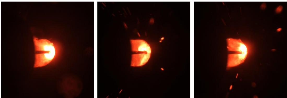
Figure S5: Test images at three typical moments under the process conditions of 145A, 21V, and 29cm/min.
