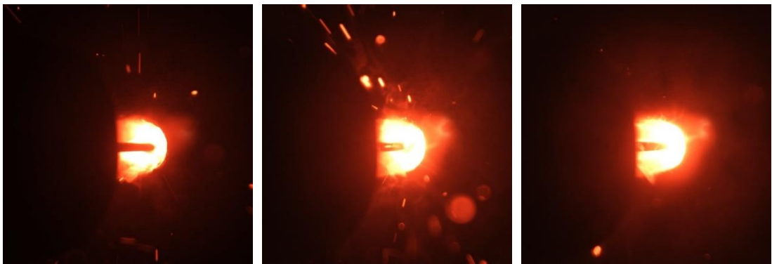
Figure S2: Test images at three typical moments under the process conditions of 95A, 19V, and 26cm/min.
