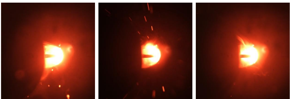
Figure S3: Test images at three typical moments under the process conditions of 125A, 19V, and 26cm/min.
