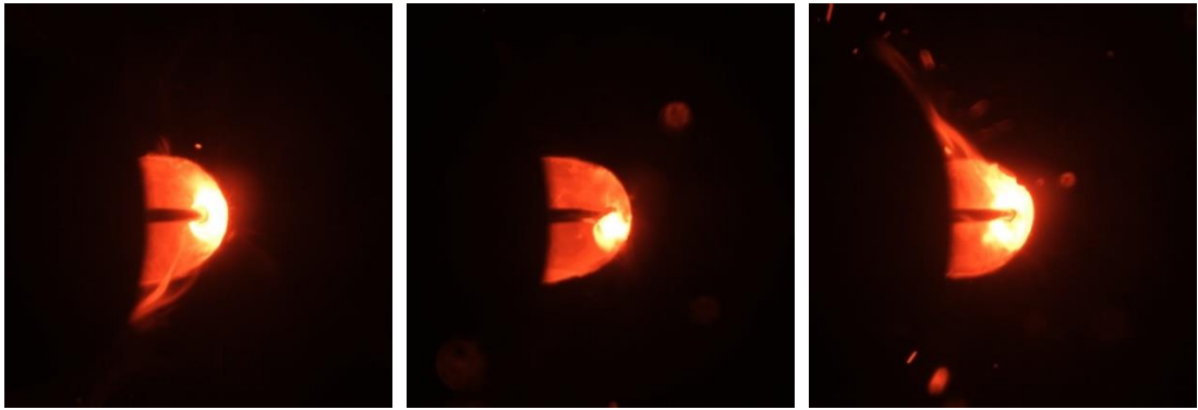
Figure S4: Test images at three typical moments under the process conditions of 125A, 23V, and 23cm/min.
