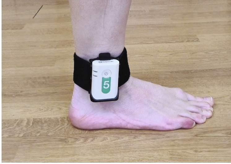
FIGURE 1: Sensor placement on the shanks using elastic straps.
