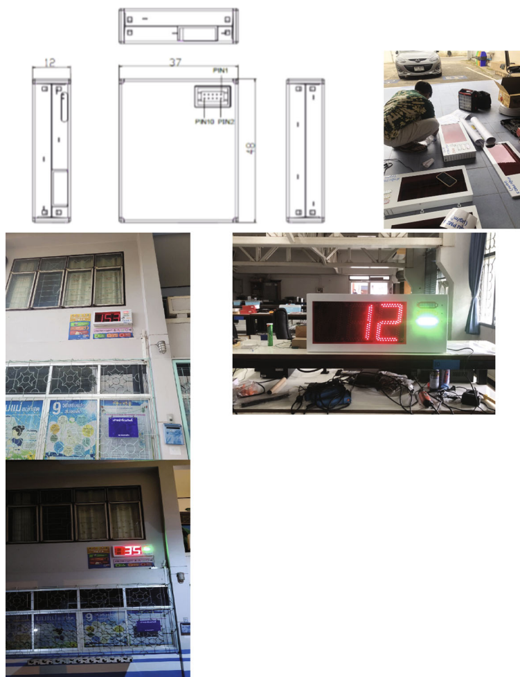
FIGURE 3: The sensor used to measure dust up to 2.5 microns in size according to this invention.
