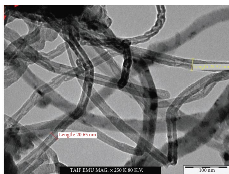
FIGURE 3: TEM image of carbon nanotube.
