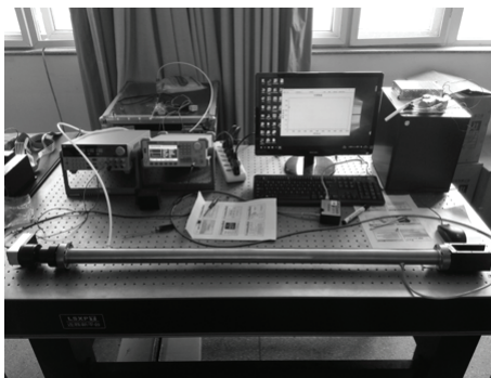
(a) Photo of the experimental system with 100 cm gas chamber
