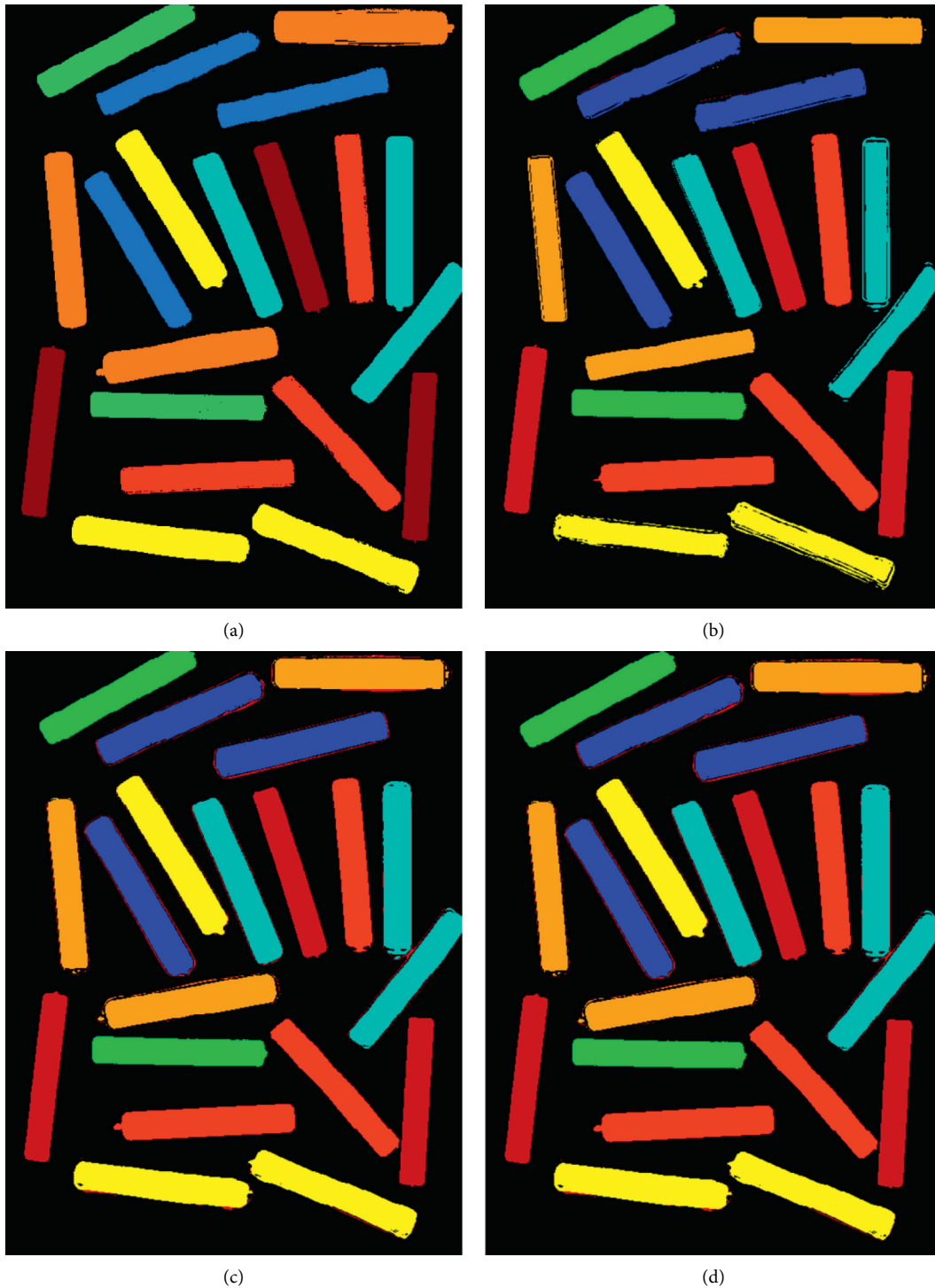
FIGURE 19: Classification results using the (a) proposed shape-based method; SVM with (b) RBF kernel, C-value of 1, and classification threshold of 0.5; (c) linear kernel, C-value of 1, and classification threshold of 0.3; (d) polynomial kernel, C-value of 1, and classification threshold of 0.3.
