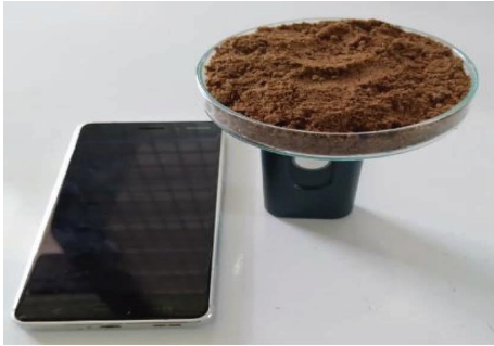
FIGURE 1: Soil spectral data acquisition setup.
