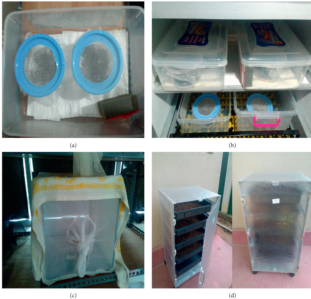
FIGURE 1: Equipment used for sand fly colony maintenance. (a) Larval rearing cups. (b) Egg laying cups and larval rearing cups placed in plastic boxes are maintained under standard conditions in an incubator. (c) Adult rearing cages made of white organdy clothes. (d) Larval food composter made for the fermentation of larval food.
