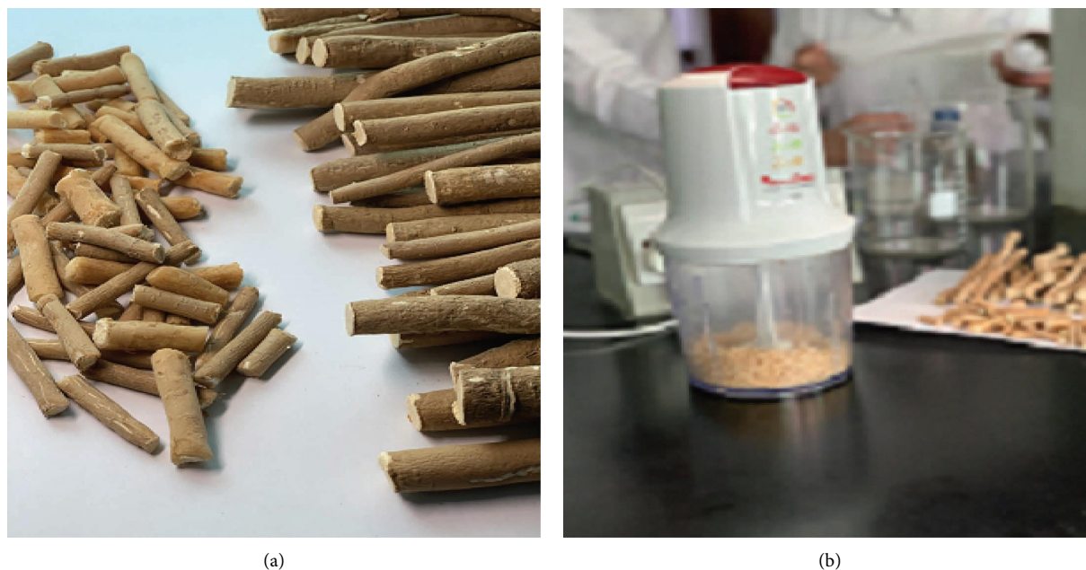
FIGURE 1: (a) Stem bark of Salvadora persica (miswak) and (b) miswak pulverised in a mechanical grinder.
