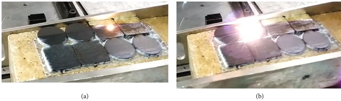
FIGURE 2: Photographs of two moments during the laser processing: (a) without coating and (b) with a C-coating. The effect of the surface state on the plasma glow could be perceived comparing (a) to (b).
