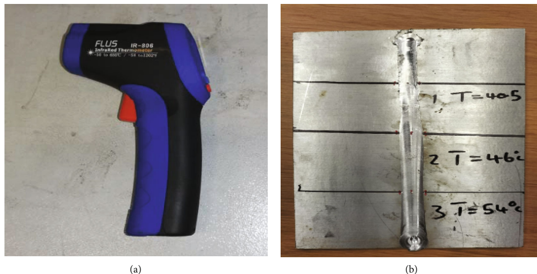
FIGURE 3: (a) Infrared thermometer. (b) Welded sample sectioned according to tool temperature.
