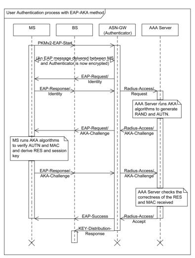
Fig. 12. The HaKMA's User Authentication process with the EAP-AKA method.
