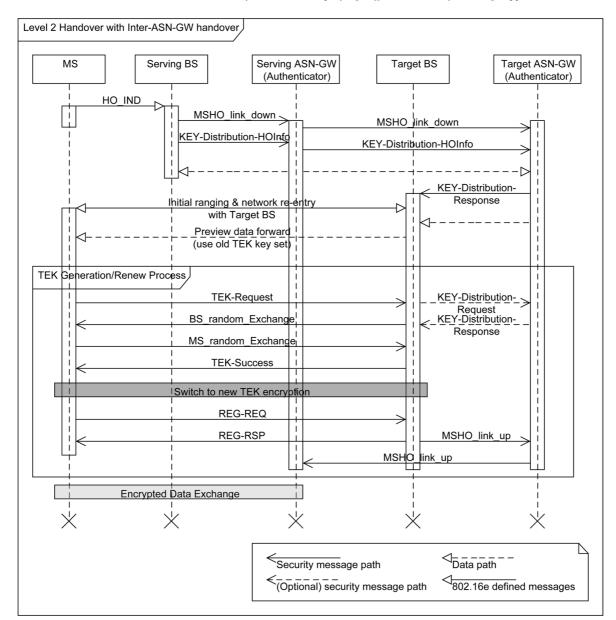
Fig. 25. The process of a Level-2 Inter-ASN-GW handover. The handover steps before the TEK Generation and Renew Process are the same as shown in Fig. 24
