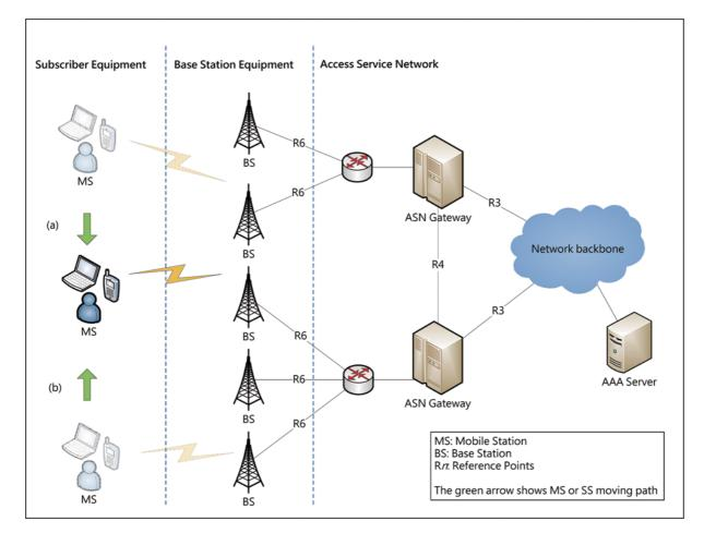
Fig. 1. The WiMax network configuration in which MS may perform an Inter-ASN-GW handover and an Intra-ASN-GW handover.
