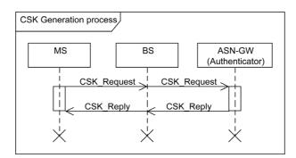
Fig. 9. Sequence chart of the CSK Generation process. BS only relays messages for MS and Authenticator.
