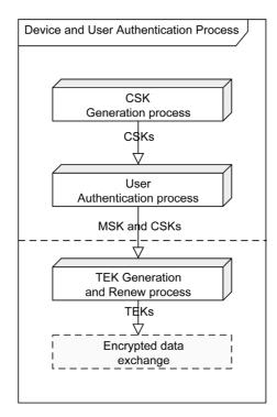
Fig. 8. Key hierarchy and sequence chart of the HaKMA authentication scheme. Processes above the dashed line are invoked by MS and Authenticator, and those beneath the dashed line are employed by MS and the BS.
