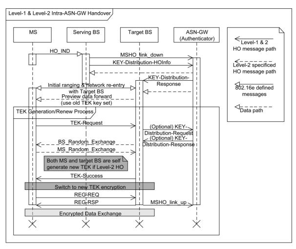
Fig. 24. The process of a Level-1 & Level-2 Intra-ASN-GW handover. The handover steps before the TEK Generation/Renew Process are the same in all Intra-ASN-GW handovers
