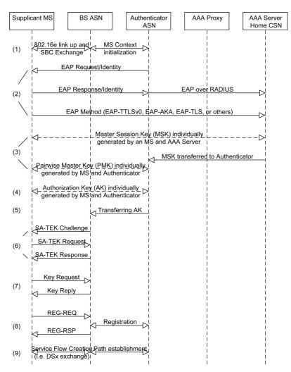
Fig. 2. The PKMv2 authentication procedure [2], where SBC stands for MS basic capability.
