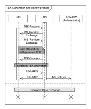
Fig. 15. Sequence chart of the TEK Generation and Renew process.
