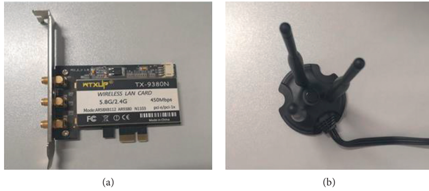
FIGURE 8: (a) WiFi commercial Atheros AR9380 NIC. (b) 5 dB high-gain external antenna.
