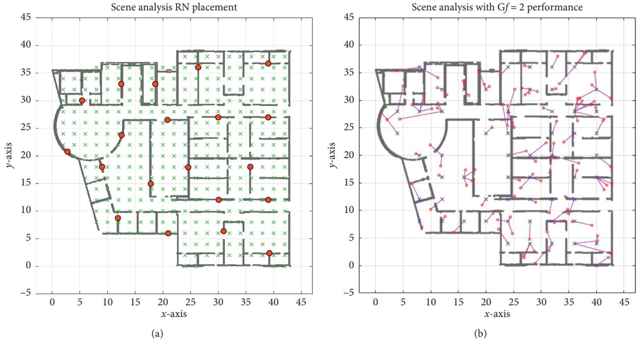
FIGURE 9: Accuracy performance of the scene analysis algorithm ( $G_f = 2$ ) with 20 RNs in Building (M). (a) RN placement obtained from the proposed framework. (b) Location performance results.
