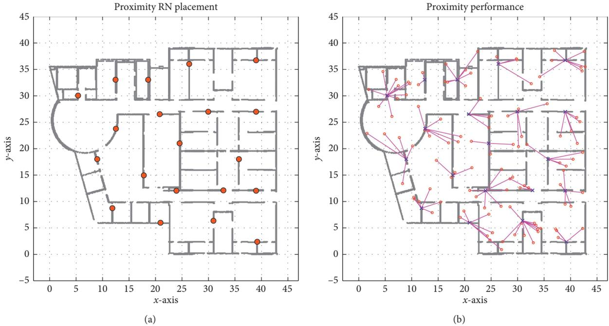
FIGURE 7: Accuracy performance of proximity algorithm with 20 RNs in Building (M). (a) RN placement obtained from the proposed framework. (b) Location performance results.
