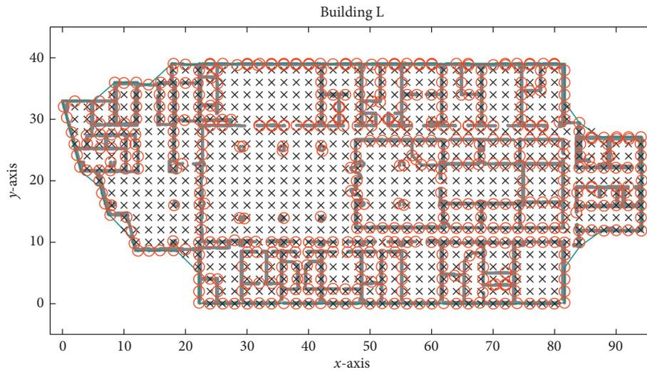
FIGURE 4: Example of candidate sites and signaling test points in auto map assignment process.
