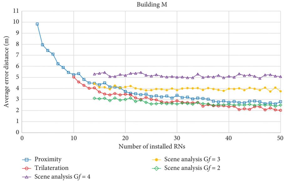
FIGURE 11: Correlation between the number of installed RNs and the average error distance for Building M.
