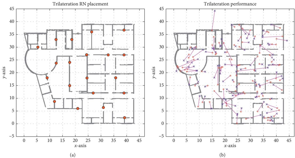
FIGURE 8: Accuracy performance of the trilateration algorithm with 20 RNs in Building (M). (a) RN placement obtained from the proposed framework. (b) Location performance results.
