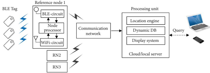
FIGURE 1: Block diagram of the main hardware components in the indoor positioning systems.
