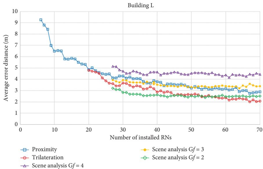
FIGURE 12: Correlation between the number of installed RNs and the average error distance for Building L.
