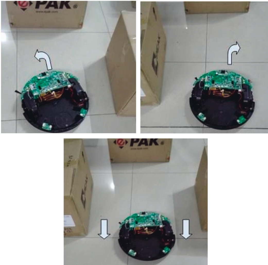
FIGURE 8: Robot path planning trend under the multidirectional obstacle environment.
