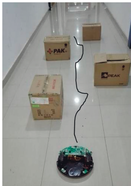
FIGURE 9: Obstacle environment in the complex environment robot path planning trend under this algorithm.
