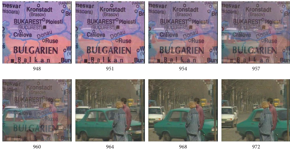
FIGURE 2: Frames of gradual transition (dissolve type).
