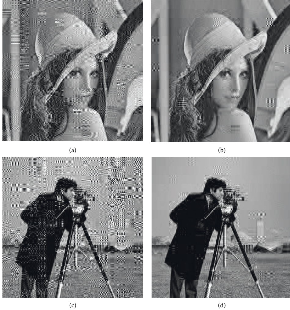
FIGURE 10: Reconstructed images at SNR of 17 dB. (a) Reconstructed “Lena” image without bit XOR. (b) Reconstructed “Lena” image with bit XOR. (c) Reconstructed “Cameraman” image without bit XOR. (d) Reconstructed “Cameraman” image with bit XOR.
