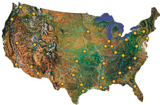
FIGURE 3: Topology of Internet2 network advanced layer 2 service.
