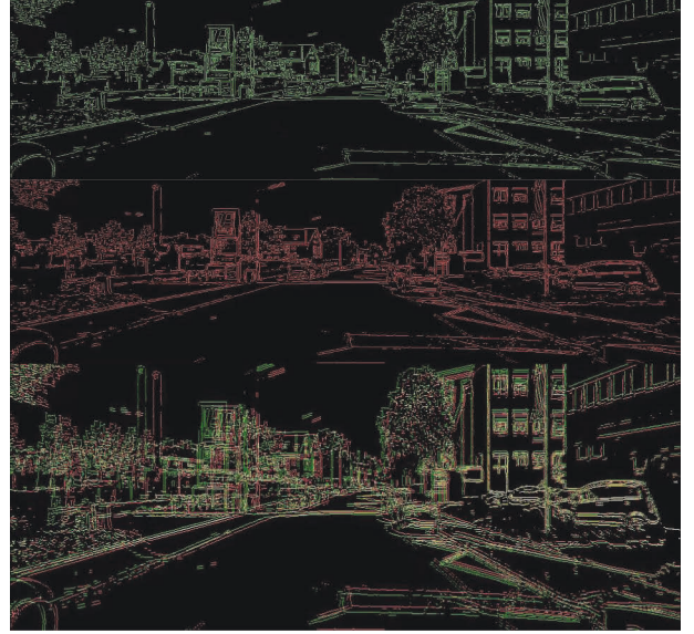
FIGURE 3: (a) The result of image edge detection after calibrating the raw image with the correct calibration parameters. (b) The result of image edge detection after calibrating the raw image with miscalibration parameters. (c) The result of overlapping the two images, you can see that the position of the corresponding pixel points in the two images has changed.
