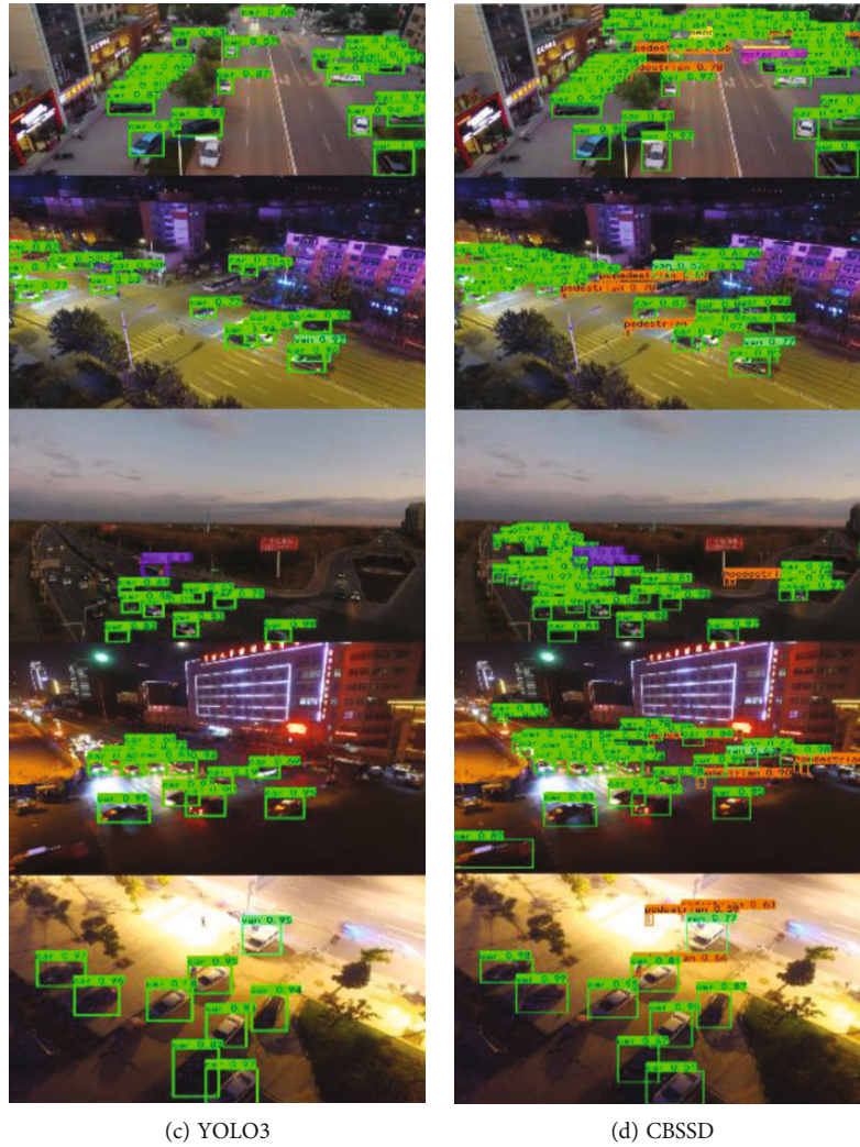
FIGURE 8: Comparison of low-illumination detection effect between CBSSD and classical object detection algorithm.
