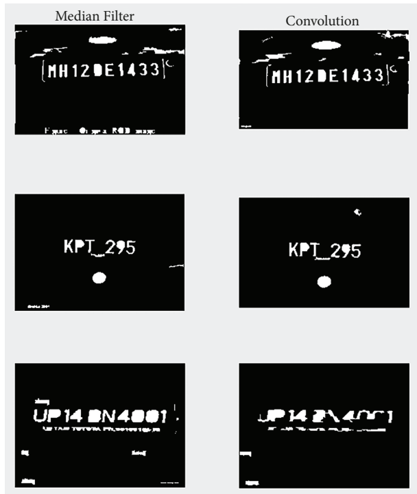
FIGURE 4: Convolution and median filter results for western number plates.
