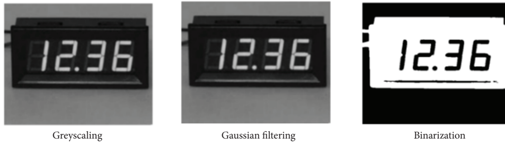
FIGURE 10: Digital meter image processing.
