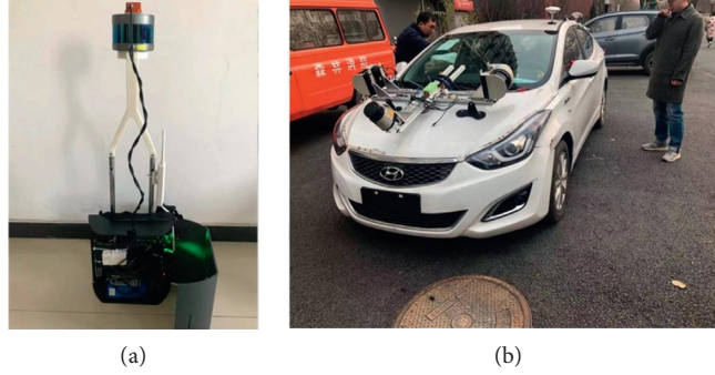
FIGURE 5: (a) backpack laser scanning equipment; (b) vehicle laser slam equipment.
