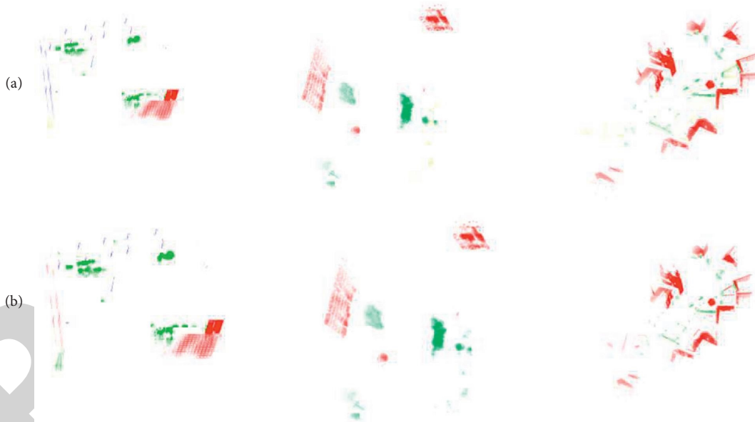
FIGURE 9: Examples of pointLAE semantic segmentation visualization on the MVFCNN dataset. (a) RGB point clouds; (b) prediction of semantic segmentation, and different colors represent different features.
