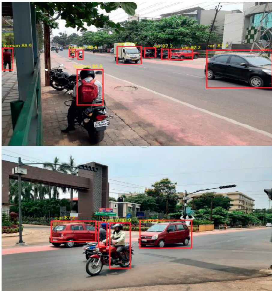
FIGURE 8: Sample outdoor obstacle detection with the SSD model.
