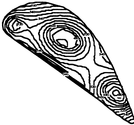
FIGURE 7(a) Temperature distribution for the reference blade.
