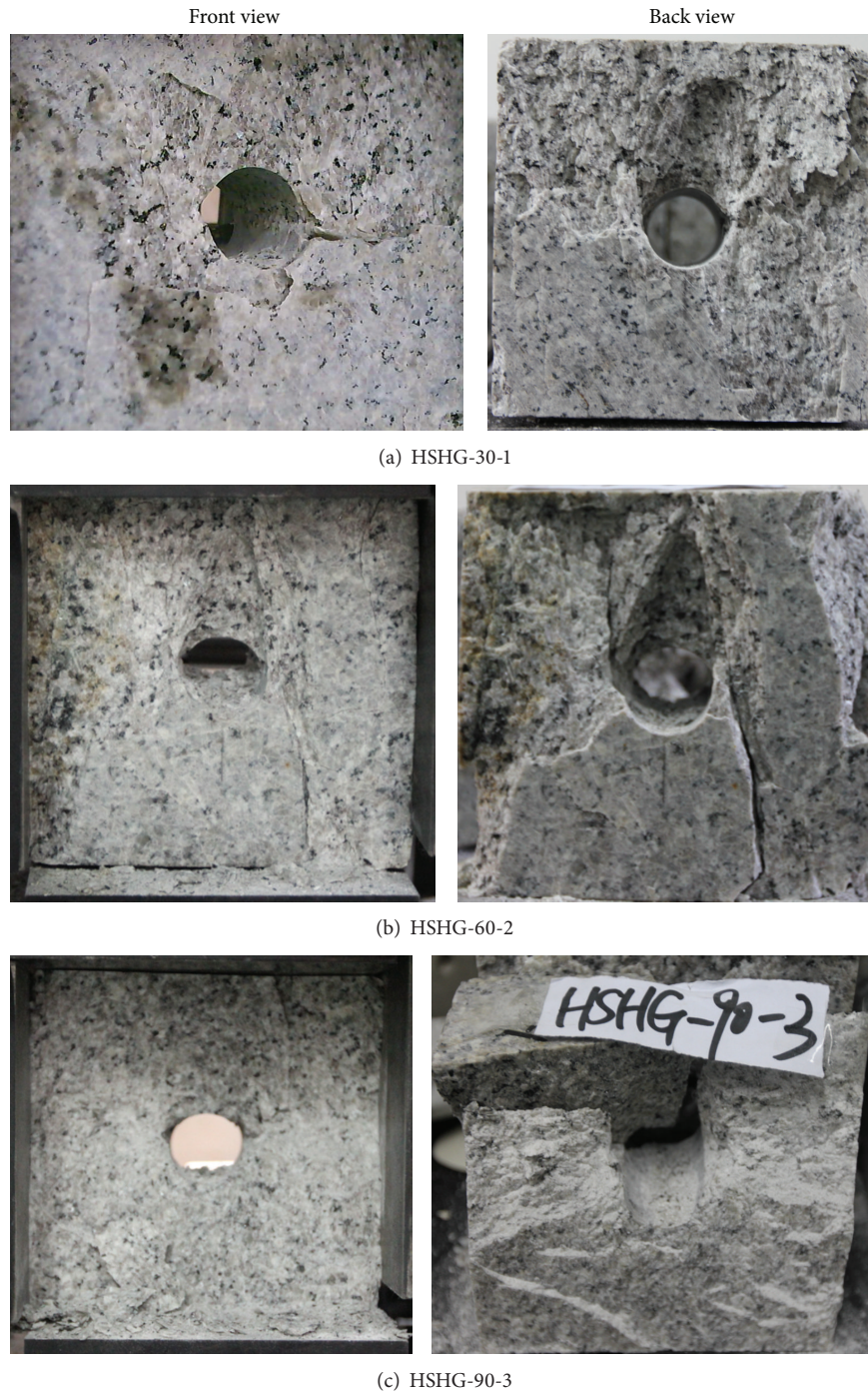
FIGURE 3: The macroscopic fracture pictures of the granite specimens.
