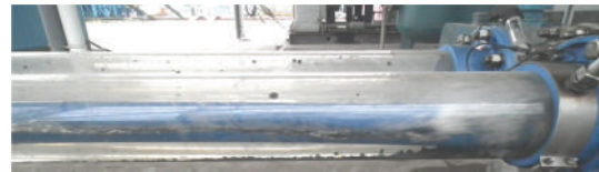
FIGURE 12: The formation of the cuttings bed.
