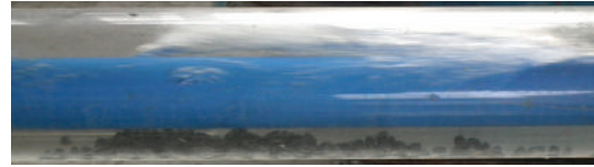
FIGURE 9: The formation of the cuttings bed.
