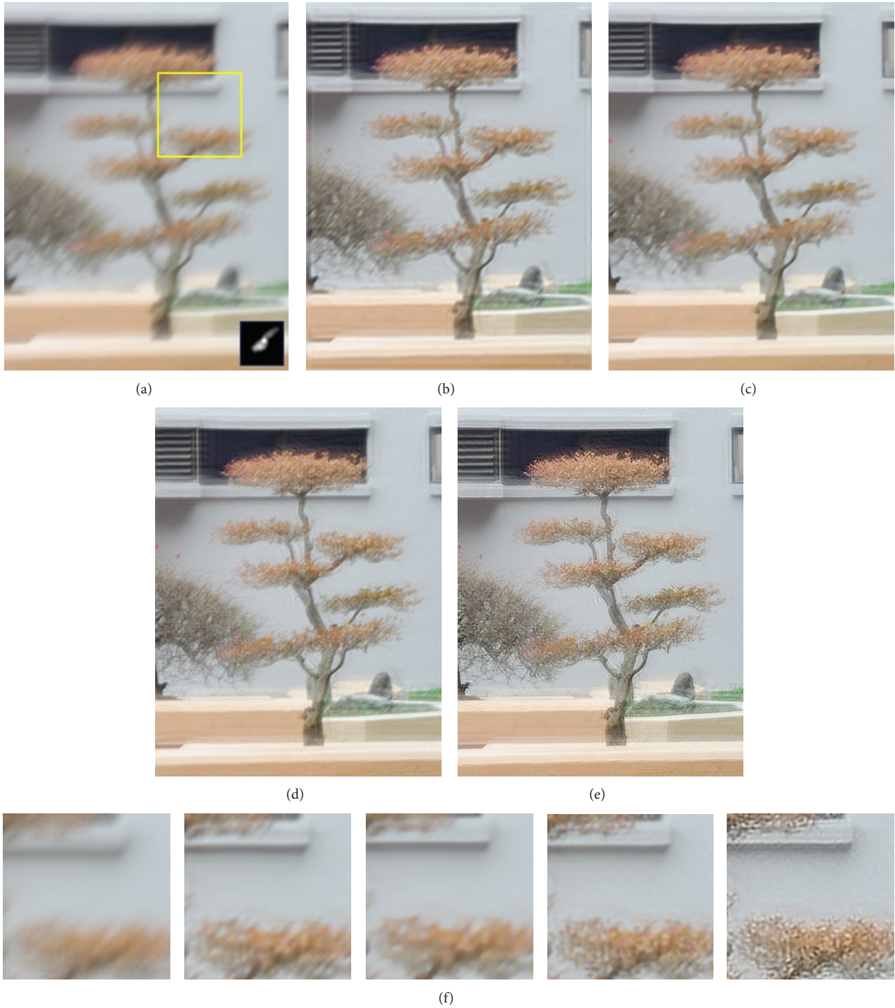
FIGURE 5: Deblurring results of real photo “Red tree.” (a) The size of blurred image is 454 \times 588 , and the estimated PSF size is 27 \times 27 . (b) The standard Richardson-Lucy method. (c) The result of Levin’s method [5] with the sparse prior. (d) The result of Krishnan’s method [7]. (e) The result of our deconvolution with adaptive regularization. (f) Close-ups of (a)–(e) image regions for comparison.
