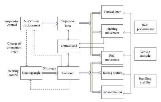
FIGURE 4: Interaction between the suspension and steering systems.
