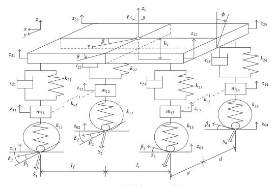
FIGURE 1: Vehicle dynamics model.
