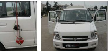
(a) Speed sensors installed on the vehicle
