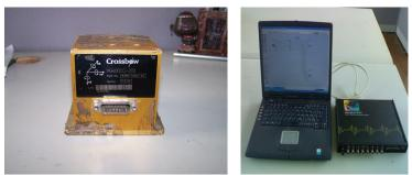
(c) Gyroscope(d) Data acquisition boxFIGURE 15: Main parts of the test and control systems.
