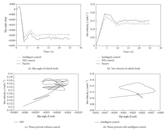
FIGURE 16: Vehicle results for angle step steering input.
