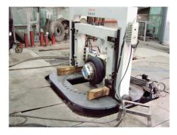
FIGURE 2: Analytical tire contact system.
