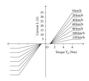
FIGURE 8: Characteristics of a linear assist.
