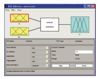
FIGURE 10: Fuzzy controller interface in Matlab/Simulink.
