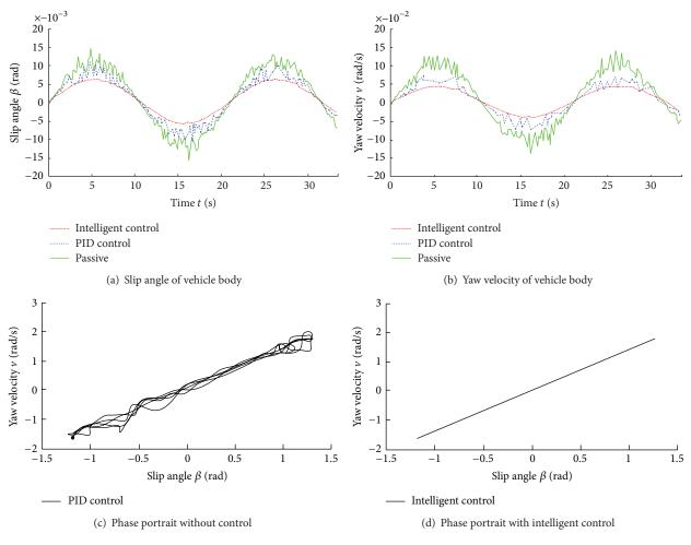
FIGURE 17: Vehicle results for S-shaped input.
