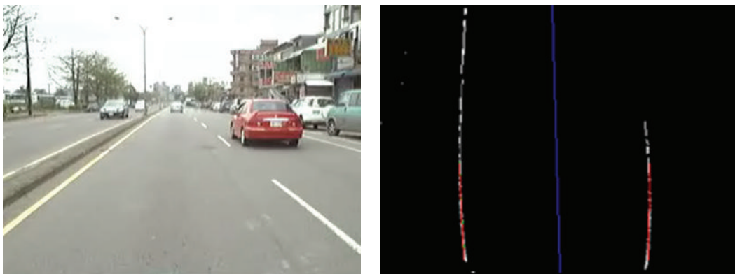
(b) Road image and detection of lane boundaries and center
