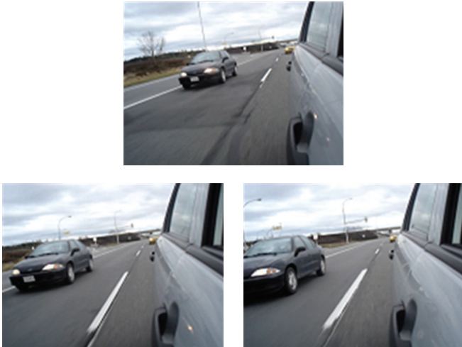
FIGURE 11: Sequence of a vehicle passing through the blind-spot region.
