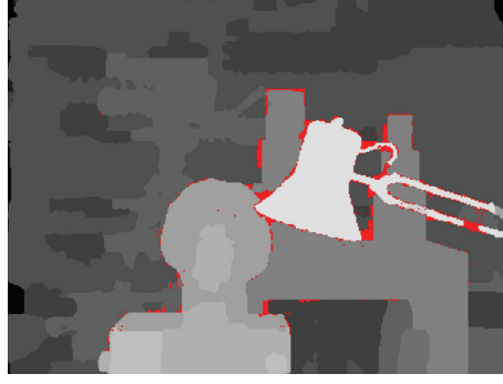
FIGURE 9: The disparity map of Tsukuba obtained by segmentation voting.
