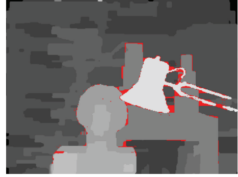
FIGURE 17: Erroneous disparity distribution after executing standard LRC checking for Tsukuba.
