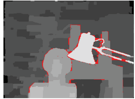
FIGURE 7: The disparity map after execution of left-right consistency checking.
