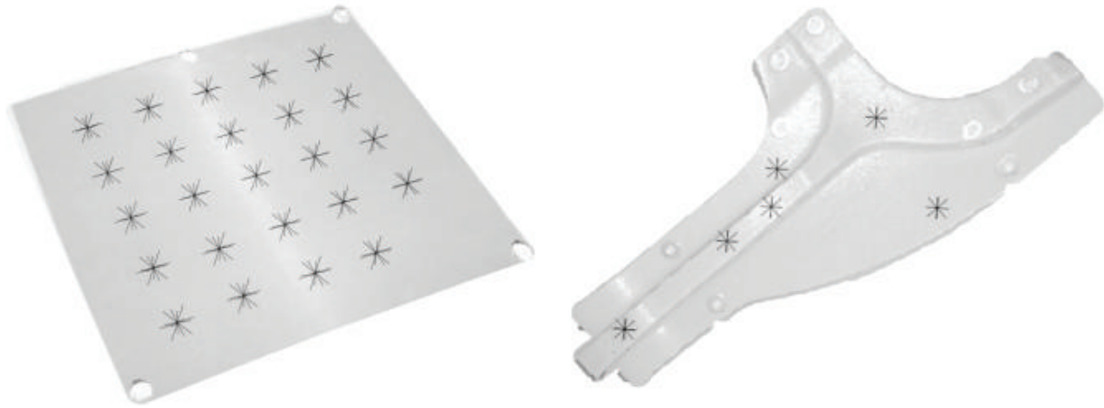
FIGURE 10: Examples of estimated position of the defects overlaid on the 3D data.
