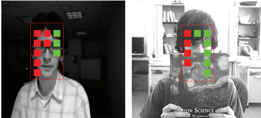
FIGURE 3: Illustration of fused weight of the ORB feature and Haar feature (video source: David video sequences and FaceOcc2 video sequences [33]).
